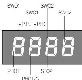
One segment of the display is linked to each input. In the event of failure it switches on according to the following scheme.
