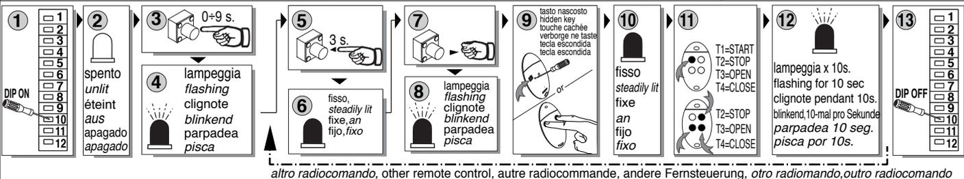
PROGRAMMAZIONE TRASMETTITORI REMOTA, REMOTE TRANSMITTER PROGRAMMING, PROGRAMMATION ÉMETTEURS A DISTANCE, FERNPROGRAMMIERUNG DER SENDER, PROGRAMACION DE TRANSMISORES REMOTA, PROGRAMAÇÃO REMOTA DOS TRANSMISORES.
